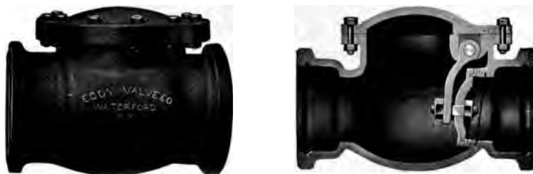
FIG. 124. — Eddy Check-valve.
